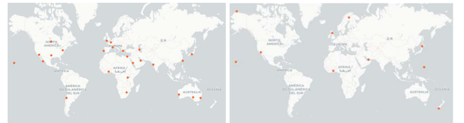
Fig. 5. 25 OGS ground network resulting from the optimization process (left) and comparative ground network for the RF X-band segment (right)
