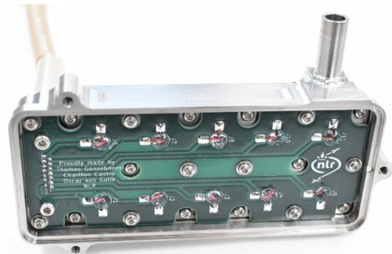
Figure 6. miniMPL Flight Model pump fully assembled except for the lid. Clearly visible are the wires connecting the piezo elements to the PCB.
