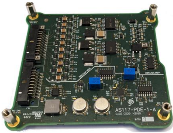
Figure 11. miniMPL Engineering Model PCB [5]. For the Flight Model the adjustable resistors (blue) and silkscreen are removed and a layer of conformal coating is applied.
