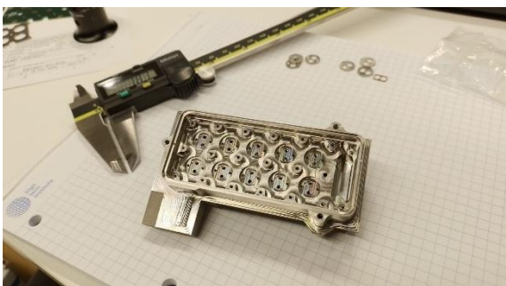
Figure 4. miniMPL Flight Model pump block during machining into final geometry.
