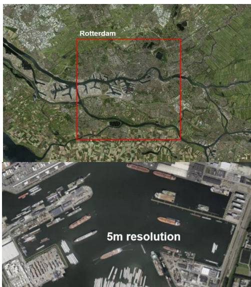
Fig 3. The Field of View from Low Earth Orbit is 25 x 25km at 500km altitude. The achievable resolution of the Tiny Telescope Model TT240-40 is 6 meters in green and 5 meters in blue wavelengths, allowing basically to observe even small boats in the harbor.
