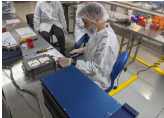
Figure 2. GigRouter connectorization prior to integration into MISSE 21 launch container (blue, foreground). [1]
