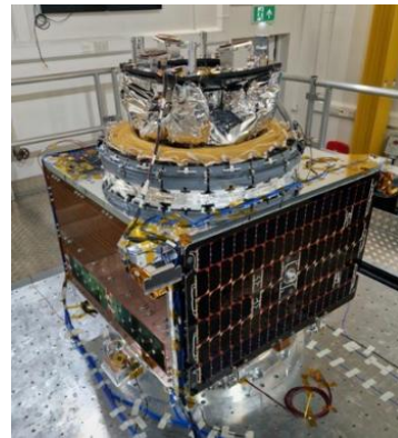
Fig. 3. CarbSAR spacecraft with stowed 3m WRA PFM mounted on earth facing panel (credit SSTL)
