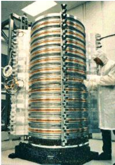
Figure 2. Alpha laser gain generator: the first MW class chemical laser demonstrated for space applications in the '90s [37].
