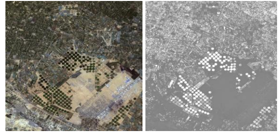
Fig. 16. Landsat-9 RGB image (left) and emissivity estimate based on NDVI (right)
