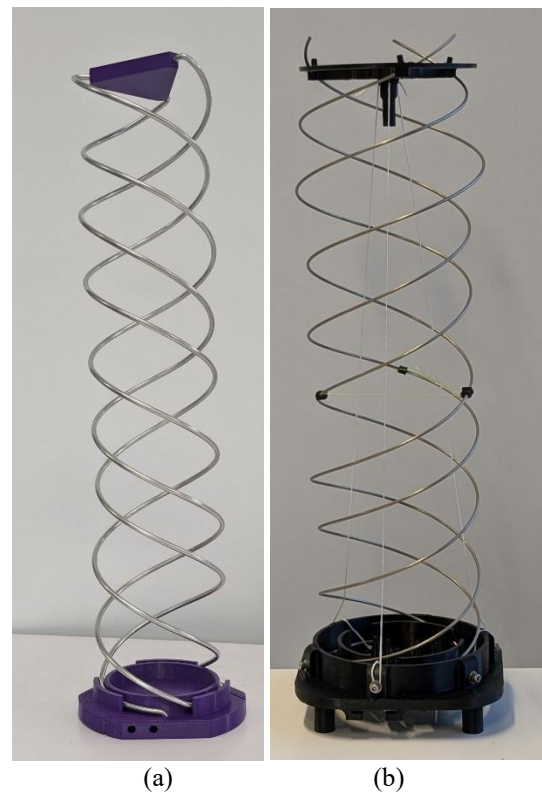
Figure 7 Antenna prototypes: (a) Aluminium wire. (b) Steel wire.
