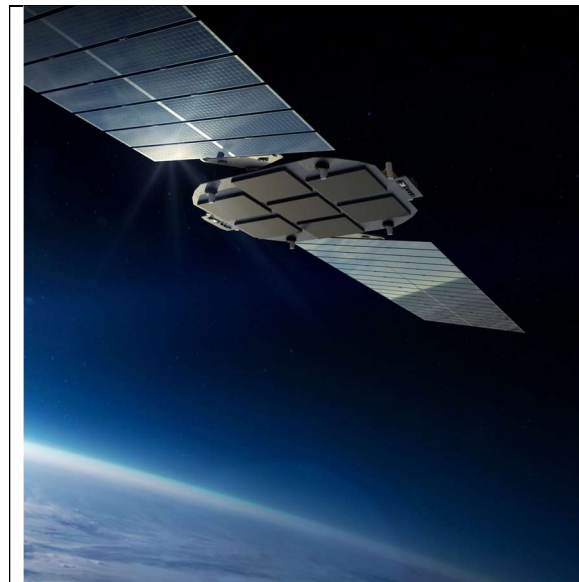
Fig. 2. Flatellite design for constellations
