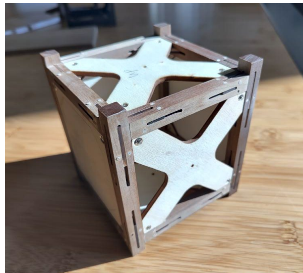
Figure 6: 1U CubeSat all wood structure - technology demonstrator
