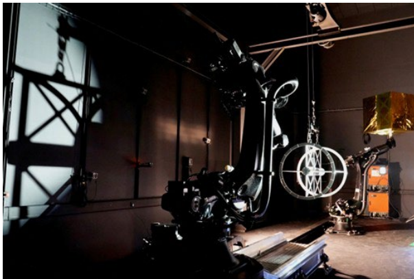
Figure 4 – Catapult RPO facility showing servicer interaction with a representative target spacecraft
