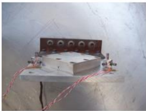
Detonation cord on back side of plate
